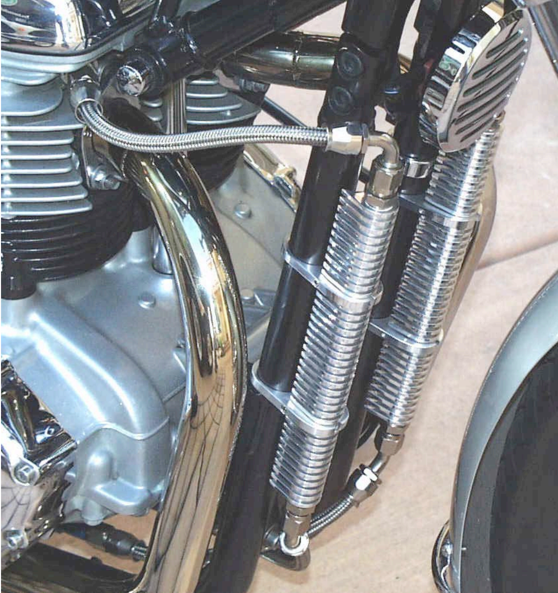
Photo #2 2001 BONNEVILLE with BP Oil Cooler Kit Installed
